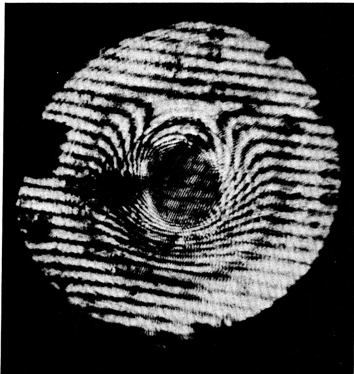
FIGURE 8. Holographic interferographic picture 350 ns after start of the current; tube radius 1 cm, length 5 cm, fill pressure 350 mTorr H_2 , current 80 kA.
